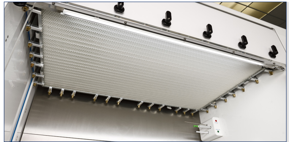
HEPA Filter located in the chamber ceiling
